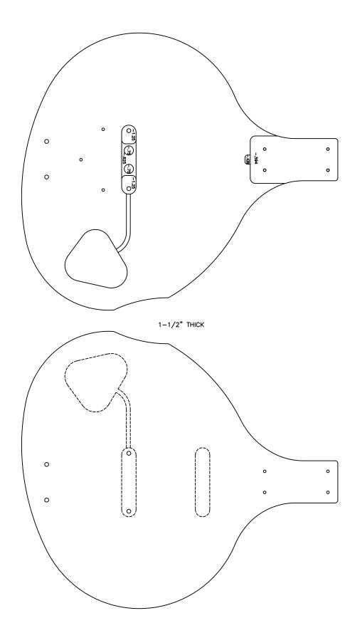
2 —— 1/8" CUTTER TO .25" DEPTH 3 — 1/8" CUTTER TO .75" DEPTH
