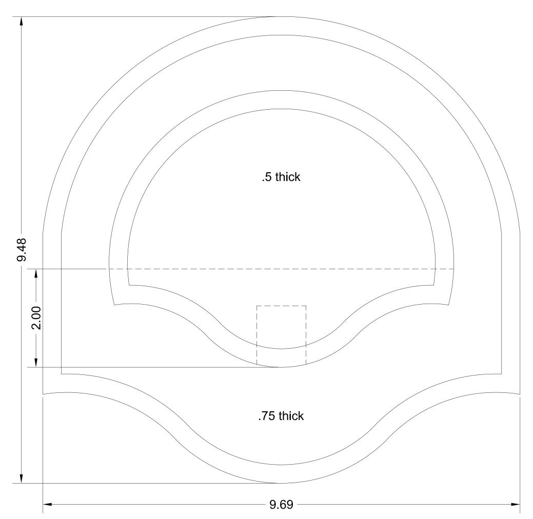
The thickness of the spacer should be the thickest part of your turkey fan plus 1/4"
