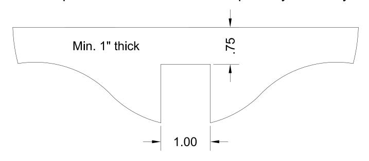
The 1.00 wide dimension for the beard notch can be narrower for a smaller beard
